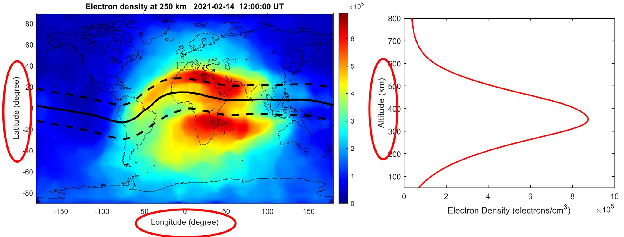
In our context, the 3-D ionospheric model involves representation of the ionosphere (electron densities) in 3 space dimensions of Longitude, Latitude, and Altitude.
