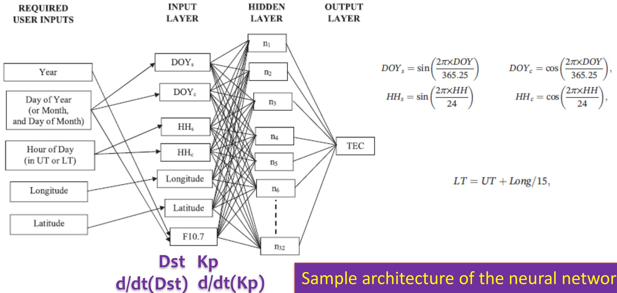
Sample architecture of the neural network model implemented in this work
