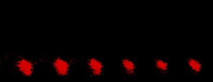
Ions levitating above the surface of a silicon microchip can move around the quantum computer and interact.
