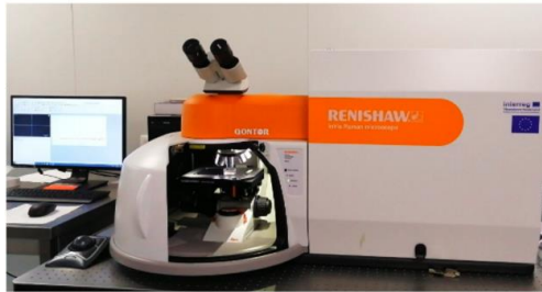
Raman spectroscopy: Identification of microplastics
