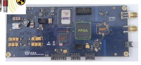
**Ionization Radiation Measurement** (FPGA-uC)
