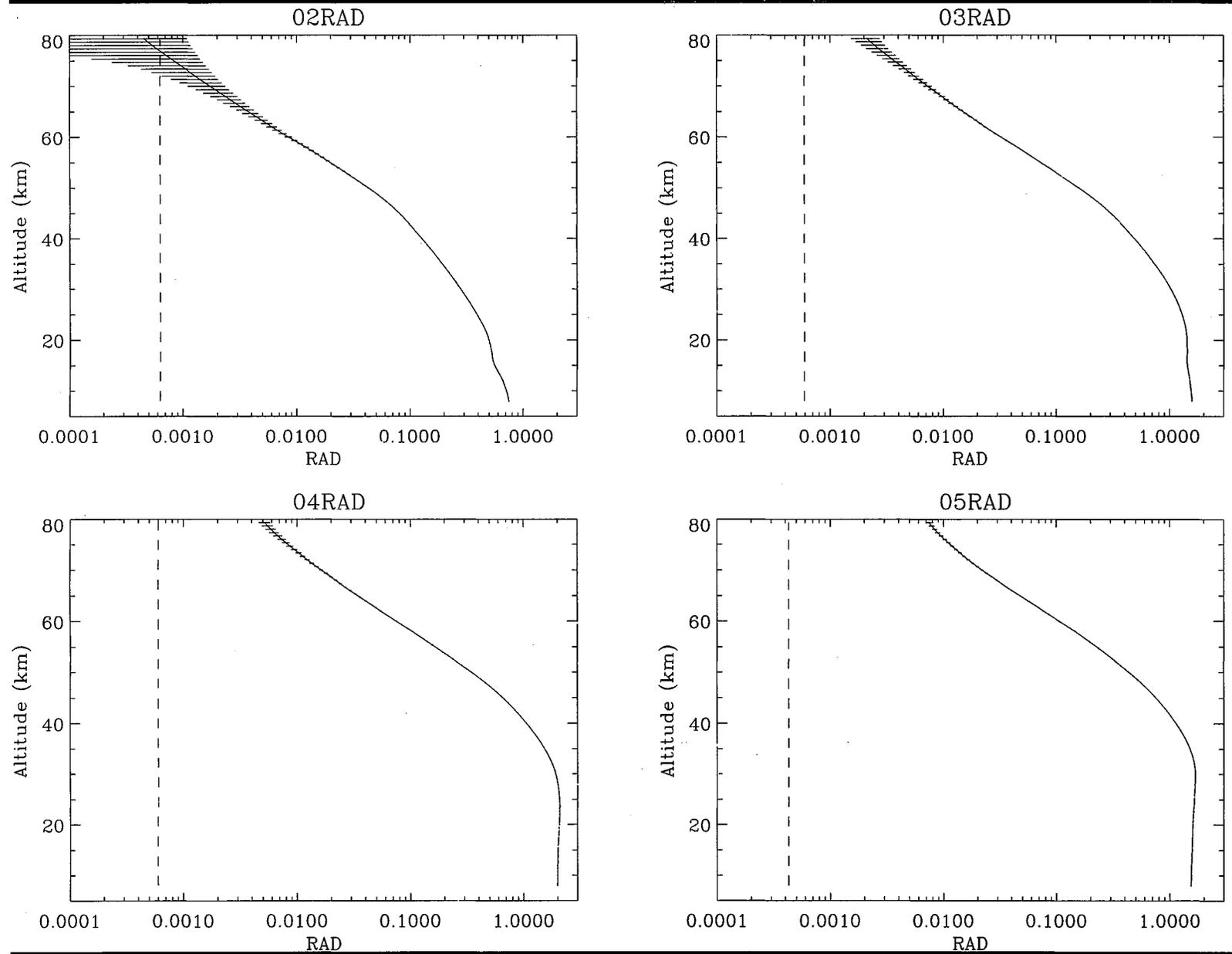
Weighting functions,  $\partial R/\partial T$ , for the HIRDLS temperature sounding channels
