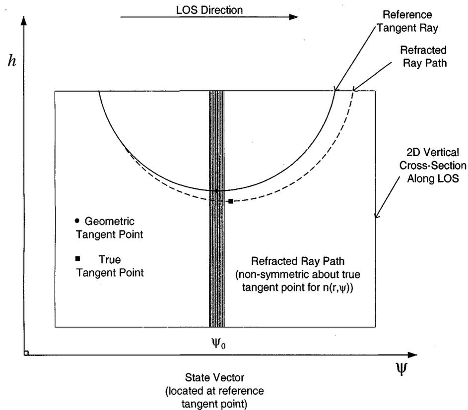
Temperature, Pressure, H<sub>2</sub>O in vertical plane along LOS are used to calculate the Refractive Index of Air and derivatives.
