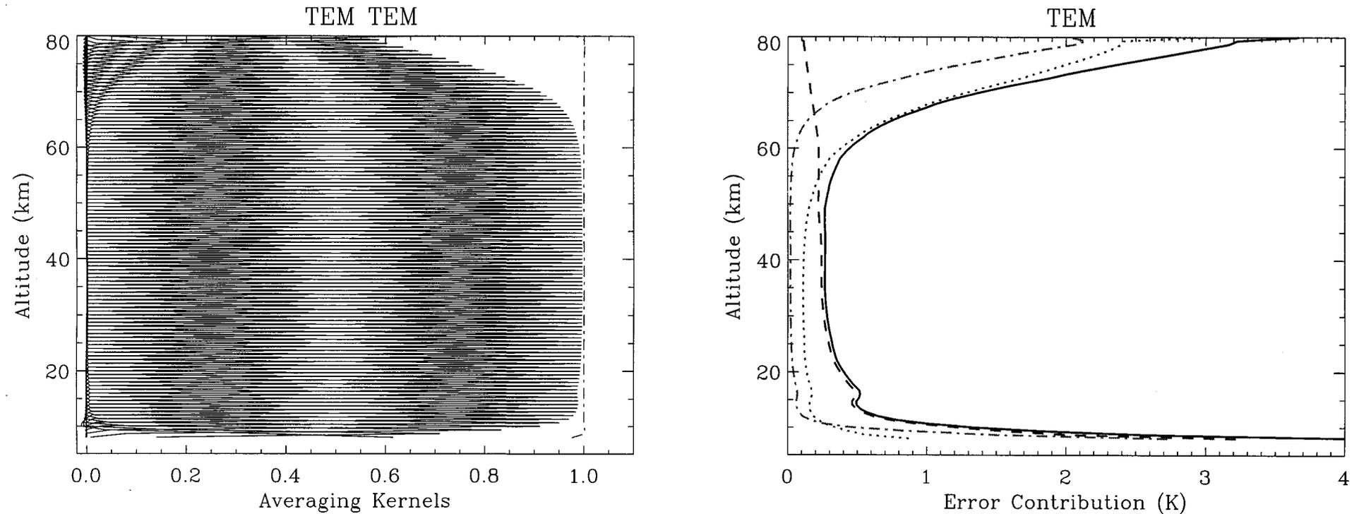
(a) Averaging kernels and (b) random error contributions for the HIRDLS temperature sounding channels calculated for the AFGL tropical atmosphere. The dot-dash line in (a) represents the sum of the averaging kernel rows. In (b) the solid line represents the total error and the dotted, dashed and dot-dashed lines represent the measurement noise, forward model and *a priori* error contributions, respectively.
