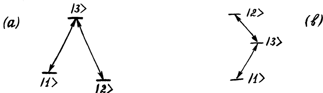
Fig.11. \Lambda (a) and cascade (b) systems of electric dipole transitions |1\rangle - |3\rangle and |3\rangle - |2\rangle between quantum levels |1\rangle , |2\rangle and |3\rangle .
