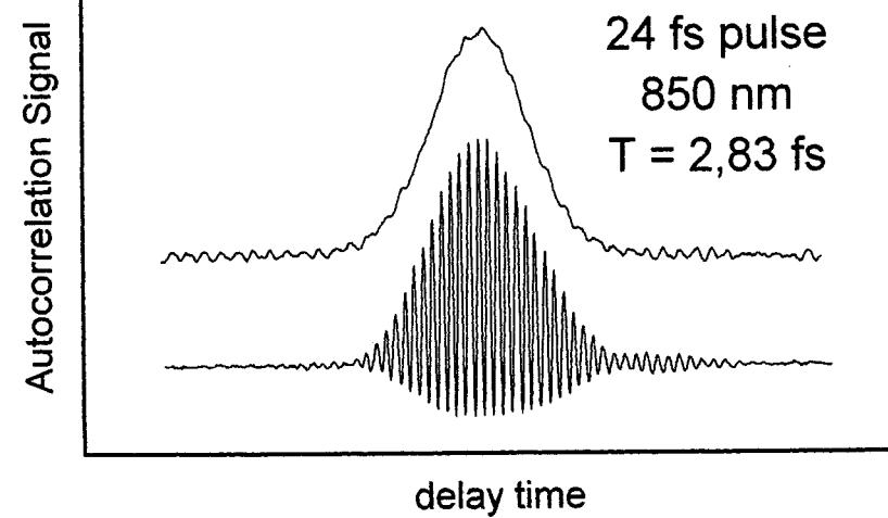
In a Michelson interferometer (with second harmonic detection) there is no complete averaging and the phase of the electric field has be taken into account:
