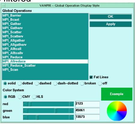
The display style can be adapted for each collective operation
