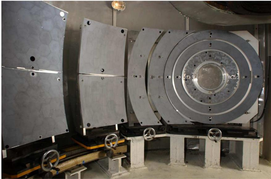
**Only the neutrons which fulfill the Bragg condition a second time (at the analyzers) are detected!**
