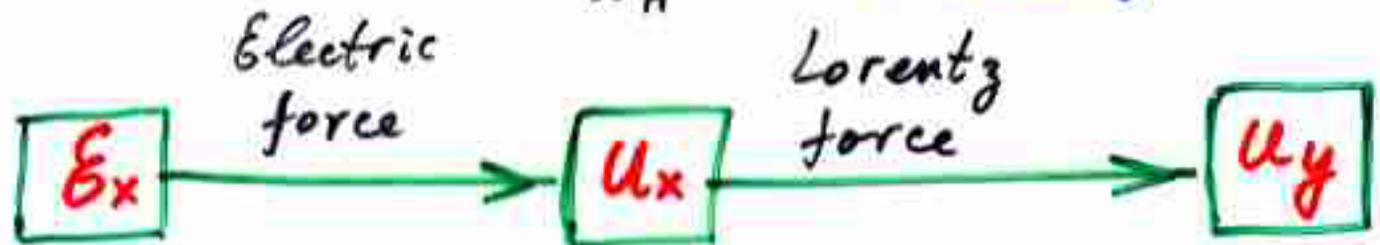
$$E_x \frac{e/m}{-i\omega + \gamma} = u_x; \quad u_x \frac{\omega_H}{-i\omega + \gamma} = u_y$$
