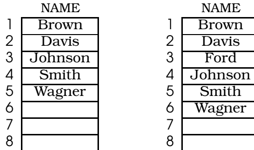
Figure 1.3: Insertion of an element in an array.
