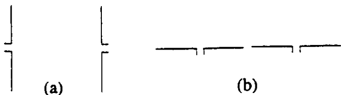
Figure 3. Half-wave dipoles spaced by \lambda/2 ; (a) side by side and (b) collinear.
