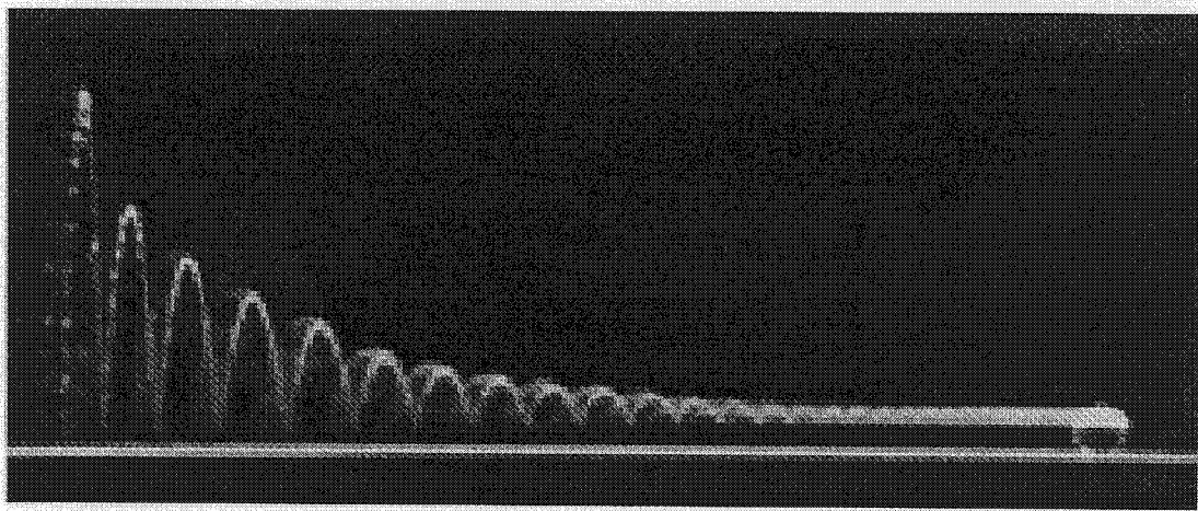
Water drop falling on a super-hydrophobic surface ( $\theta = 170^\circ$ ) of very small contact angle
