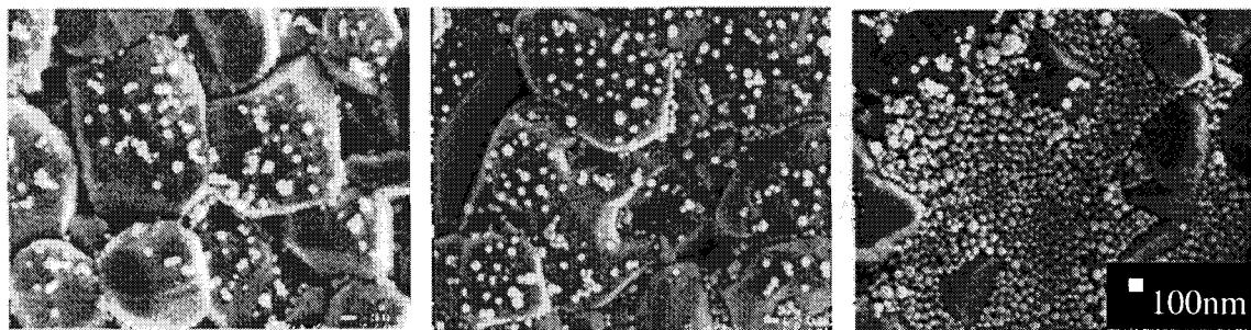
Silica particles ( $\approx 45$  nm in diameter) adsorbed onto the surface of polycrystalline alumina substrates.
