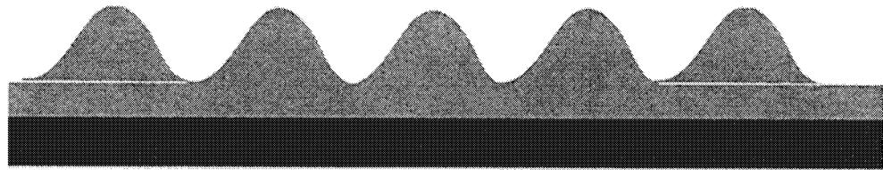
**Textured, thin film produced by spin coating  $\text{Al}_2\text{O}_3$  precursor**
