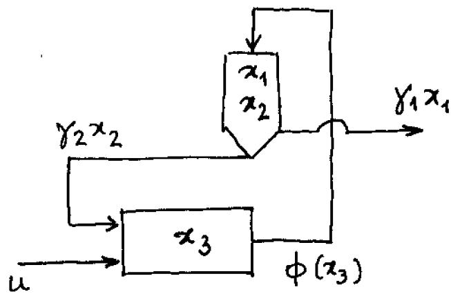
$$\begin{pmatrix} \dot{x}_1 \\ \dot{x}_2 \\ \dot{x}_3 \end{pmatrix} = \underbrace{\begin{pmatrix} 1-\alpha & 0 \\ +\alpha & -1 \\ -1 & +1 \end{pmatrix}}_{\rho(x)} \begin{pmatrix} \phi(x_3) \\ \gamma_2 x_2 \\ \gamma_1 x_1 \end{pmatrix} - \begin{pmatrix} \gamma_1 x_1 \\ 0 \\ 0 \end{pmatrix} + \begin{pmatrix} 0 \\ 0 \\ u \end{pmatrix}$$
