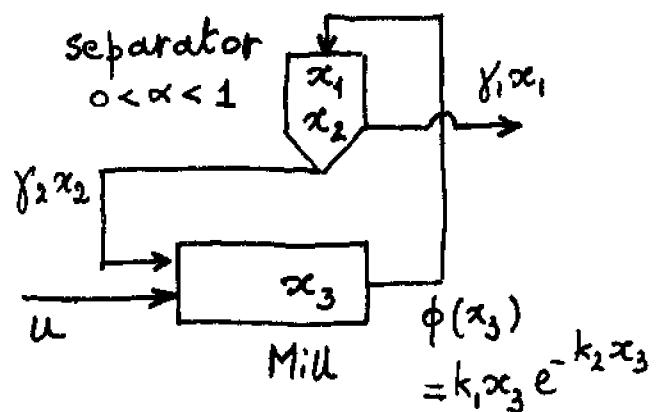
$$\begin{pmatrix} \dot{x}_1 \\ \dot{x}_2 \\ \dot{x}_3 \end{pmatrix} = \underbrace{\begin{pmatrix} (1-\alpha) \phi(x_3) \\ \alpha \phi(x_3) - y_2 x_2 \\ y_2 x_2 - \phi(x_3) \end{pmatrix}}_{n(x,u)} - \underbrace{\begin{pmatrix} y_1 x_1 \\ 0 \\ 0 \end{pmatrix}}_{q(x,u)} + \underbrace{\begin{pmatrix} 0 \\ 0 \\ u \end{pmatrix}}_{p(x,u)}$$
