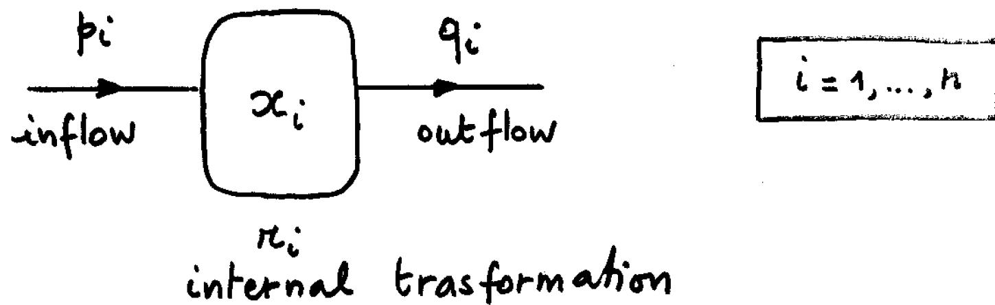
mass balance  $\dot{x}_i = r_i - q_i + p_i$
