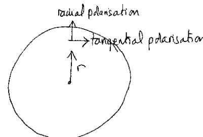
$\Delta n_r$  is the refractive index change for light polarised in a radial direction,
