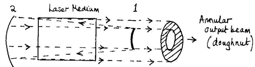
This gives a collimated beam (plane wave-front) travelling left to right. The central portion is reflected (leaving an annular output to escape around the small mirror) and the reflected portion is magnified transversely by a factor  $M$  before being converted into a uniform plane wavefront by mirror 2. If the small mirror has radius  $a_1$ , then the plane beam striking this mirror has radius  $Ma_1$ , and the fraction of power coupled out is  $1 - 1/M^2$ .
