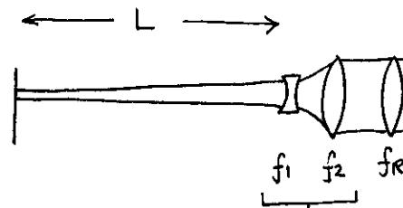
$$\text{Telescope, magnification } M = -\frac{f_2}{f_1}$$
