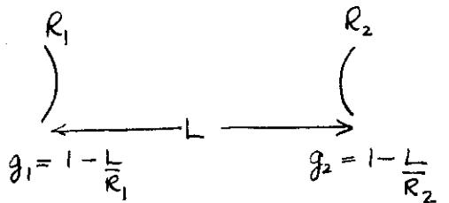
The convex-convex resonator is unstable since  $R_1, R_2 < 0$ , hence  $g_1, g_2 > 1$  and  $g_1 g_2 > 1$ . It clearly displays the characteristic of any unstable resonator, i.e. the beam passing back and forth between the mirrors progressively grows in transverse extent.
