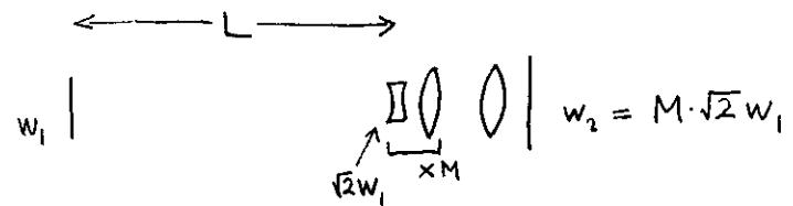
These results (10), (11) are easily remembered by thinking of the part of the resonator to the left of the telescope as acting like a half-conformal resonator; spot-size at centre of conformal resonator of length  $2L$  is given by  $w_1^2 = \frac{2L\lambda}{\pi} = \frac{L\lambda}{\pi}$ . The spot size at the input to the telescope is then  $\sqrt{2} w_1$  and after the telescope is  $M\sqrt{2} w_1$ , i.e.  $w_2^2 = 2M^2 w_1^2 = \frac{2M^2 L\lambda}{\pi}$
