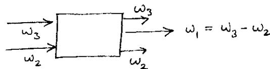
Assume input waves to nonlinear medium at frequencies  $\omega_3$  and  $\omega_2$ . A wave at the difference frequency  $\omega_1 = \omega_3 - \omega_2$  is generated.
