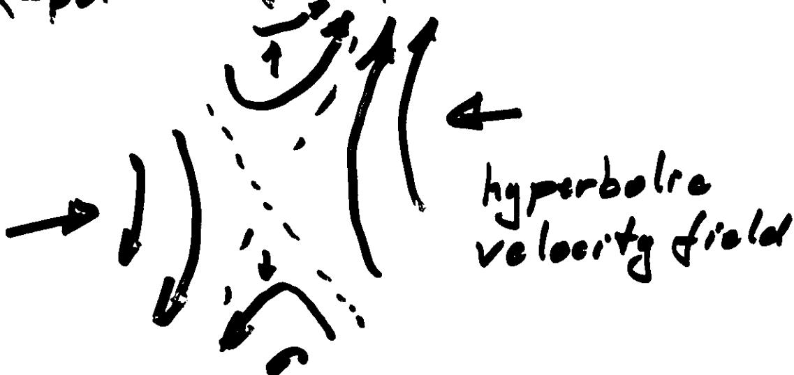
neutral line is a degenerate case - current density around the X-point
