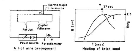
Acalorimeter method<sup>4</sup> for finding diffusivity ( $\alpha_e$ ) — This method is based on the theory of heating a soil sample encased in a metallic container in the stage of regular thermal regime. Knowing shape factor B of the test body, which in case of cylindrical containers depend on radius r and length 1, and by slop of log deflection versus time curve one determines diffusivity of the soil using expression
