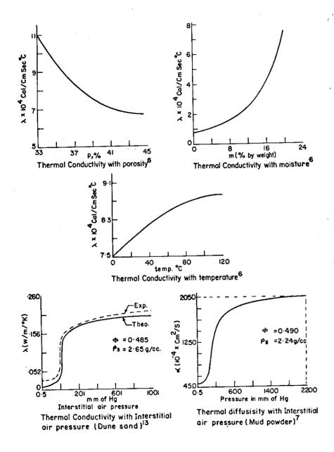
Predicting  $\lambda_e$  of two phase systems - Dry sand is considered homogeneous in respect of heat flow, which occurs on a molecular scale, and here the process effective is conduction. In such a sample heat flux density H, Quantity of heat flowing per unit time per unit of surface area, is proportional to the temperature gradient  $\nabla \theta$  (°C/cm)<sup>7</sup>.
