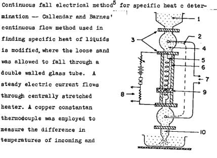
out going material. To vary rate of fall different diametered nozzles were employed. Specific heat c was calculated from  $c = (i_1^2 - i_2^2) Rx 10^7 / J(m_1 \Delta \theta_1 - m_2 \Delta \theta_2)$
