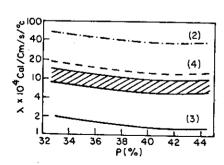
In order to obtain better results an equation analogous to (4) should be taken whose predictions fall within cross-hatched region. We considered weighted geometric mean of maximum thermal conductivity (2) calling
