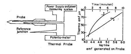
Hot wire<sup>3</sup> for determination of thermal diffusivity  $(\alpha_e)$  — When the point of observation in the sample is at a distance r from the line heat source the thermal diffusivity is determined by  $\alpha_e = r^2/4t$ , where t is the time at the point of inflection of temperature  $\theta$   $(t = t_{max})$ .
