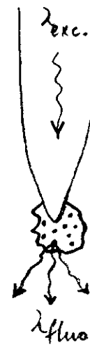
Fig.24 Schematics of the arrangement for choosing a single molecule in a small matrix as an emitter for optical near-field microscopy.
