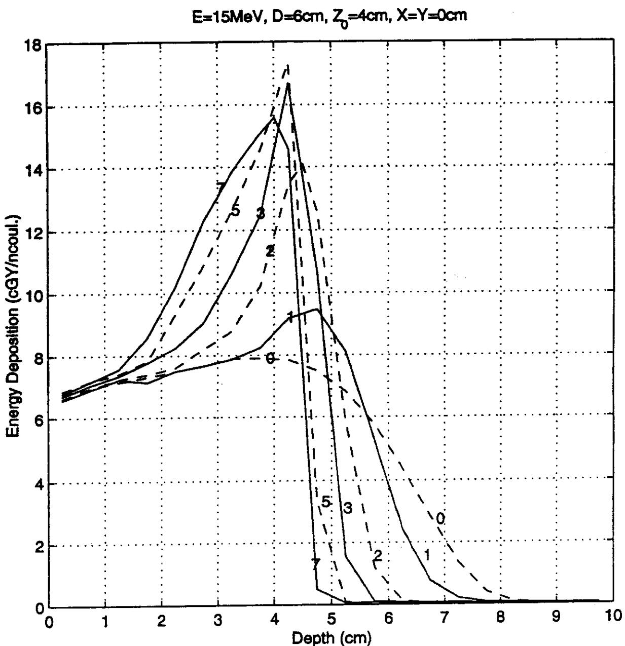
Central-axis depth-dose curves for electron beams incident with an energy of 15 MeV and a beam diameter of 6 cm. The initial 4 cm layer of tissue is field-free, after which there is applied a uniform magnetic field perpendicular to the beam axis. Results are from the ITS v. 3 Monte Carlo code ACCEPTM, and are shown for magnetic fields of 0, 1, 2, 3, 5 and 7 T. From Nardi and Barnea (1999).
