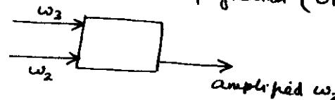
Here we consider the situation where a large amplification of  $w_2$  is achieved ( $w_3$  is a powerful pump). This can be used either as a means of amplifying a weak signal or as a means of generating a significant power at the idler frequency  $w_1 = w_3 - w_2$ . The output power at the idler is (for large gain) equal to  $\frac{w_1}{w_2}$  times the output signal power.
