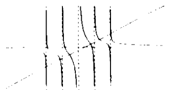
FIG. 2. Graphical solution of the eigenvector-eigenvalue equation for a (1, N) system. The eigenvalues are given by the intersection points of the straight line \lambda = \lambda with F(\lambda) .
