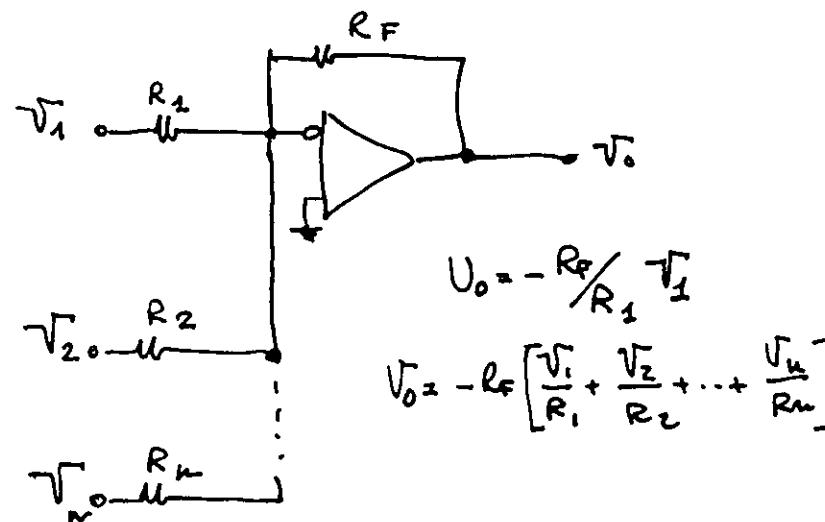
$$U_o = -R_F / R_1 V_1$$
