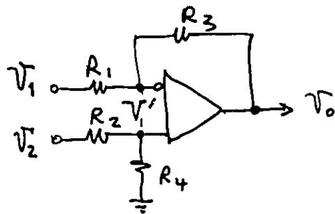
$$\text{From } V' = \frac{V_2}{R_2 + R_4} * R_4$$
