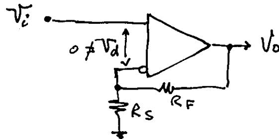
$$V_d = V_i - \frac{V_o}{R_s + R_F} \cdot R_s$$
