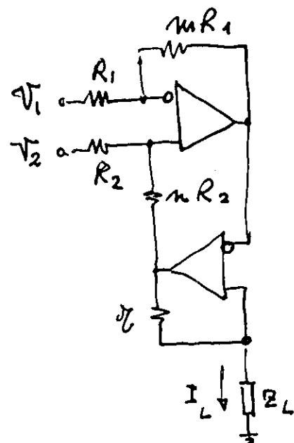
WE WANT TO MAKE A VOLTAGE ( $V_2 - V_1$ ) CURRENT GENERATOR.
