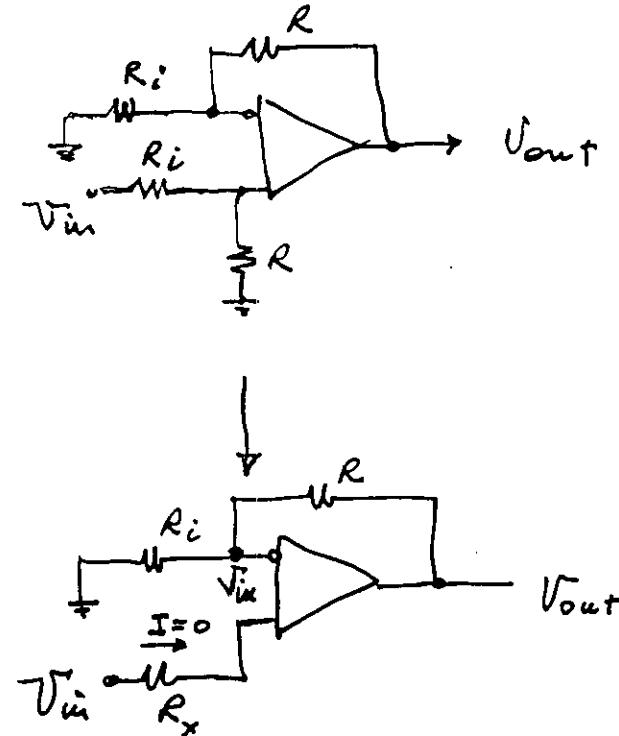
$$\frac{V_{out} - V_{in}}{R} = \frac{V_{in}}{R_i}$$
