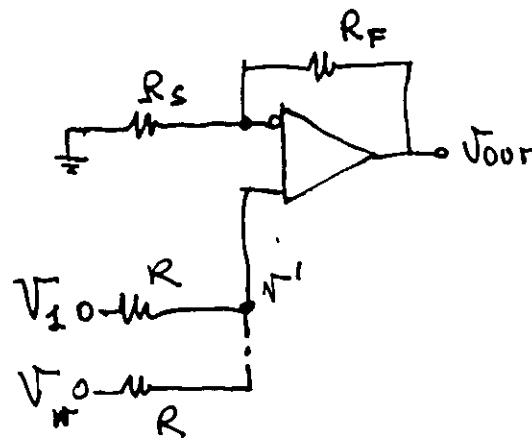
$$V'_1 = \frac{V_1}{R + \frac{R}{N-1}} \times \frac{R}{N-1} = \frac{V_1}{N}$$
