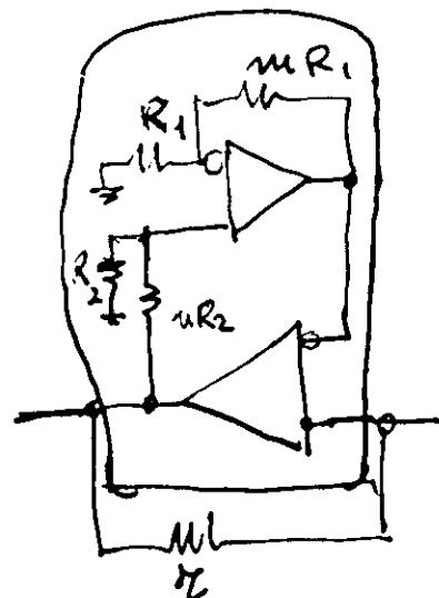
$$Z_{in} = \frac{Z_{inF} R_F}{R_F + Z_{inOL} (1 - A_{OL})}$$
