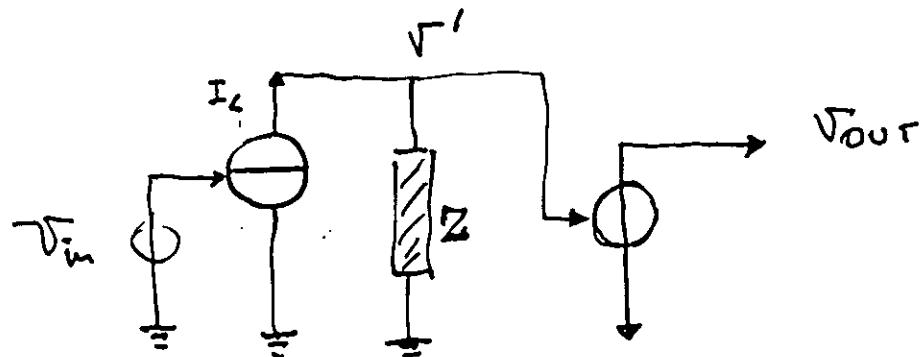
VOLTAGE CONTROLLED CURRENT GENERATOR, THAT
