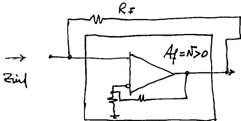
$$Z_{in} = \frac{Z_{inoc} R_F}{R_F + Z_{inoc} (1 - A_{oc})}$$
