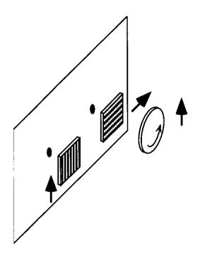
Each aperture of the Young interferometer is covered by a linear polarizer, the two polarizers being crossed. In addition one of the polarizers is followed by a  $\pi/2$  rotator so that the outcoming fields can interfere (if correlated).
