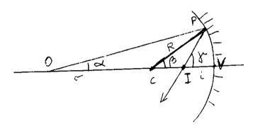
Let  $\alpha$   $\beta$  and  $\gamma$  the three angles, with respect to the axis, under which P is seen from O, C and I respectively. Note that  $\beta$  measured in radiants is given by  $\gamma$  = (arch PV)/R.
