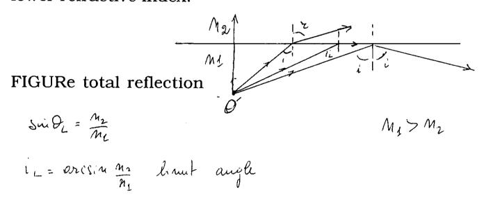
This effect finds important application in guided optical propagation (plane, or integrated optics) and optical fibers and prisms. In guided propagation it is utilized both for guiding of radiation and for coupling between fibers and other devices.
