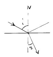
Ray from medium 1 impinges on the refracting surface at point P
