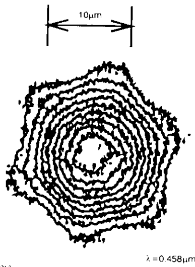
Fig. 2 Contour map of near field intensity distribution for guided mode in fibre shown in Fig. 1 at wavelength \lambda = 458 nm
