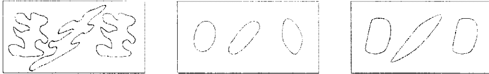
Figure 1.19: Experimental check of the affine invariance of the affine shortening (AMSS). We display on the left image three shapes. The second one is an affine transform AS of the first shape S . The third one is obtained from the second by the inverse affine transform. It therefore initially is A^{-1}AS = S . On the right image : result after application of AMSS to the two first shapes : are viewed S(t) , (AS)(t) and A^{-1}((AS)(t)) . If the numerical scheme is affine invariant, this third shape must coincide with S(t) , which is indeed the case. Middle : the same procedure applied with the curvature equation, which proves not to be affine invariant, as expected (Chapter 24).
