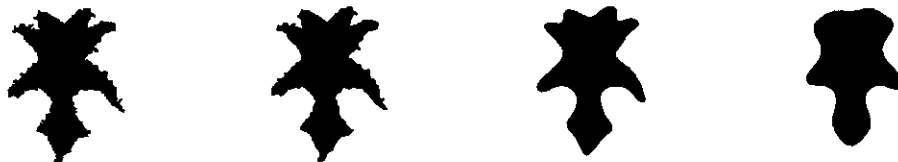
Figure 1.3: Analysis of a shape. Left: Original scanned shape, then some simplified versions: the aim here is not restoration, but analysis, that is, to define more and more sketchy versions of the shape. Those sketchy versions may permit a very short and invariant encoding of the shape. Notice how the number of inflexion points of the shape has decreased in the simplification process (Chapter 22).
