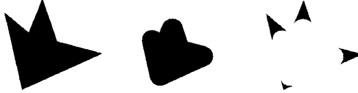
Figure 9.4: Opening of a set as curvature threshold from above. A set X , its opening by a ball of radius 20, and the difference between original and processed. This opening transforms X into the union of all balls of radius 20 contained in it. The resulting operation can be understood as a threshold from above of the curvature of the set boundary.
