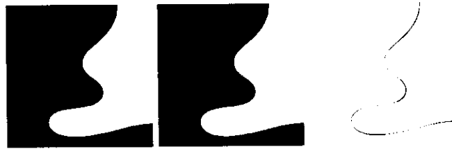
Figure 18.2: Comparison of the iterated median filter and of the curvature motion. Numerically, the iterated median filter and the curvature motion are very close, when the curvatures of the level lines are not too small. Indeed, the iterated median filter converges towards the viscosity solution of the curvature motion. Left : simple shape smoothed by a finite difference scheme of the curvature motion, middle : smoothing by a median filter at the same scale, right : difference between left and middle images. The difference is not larger than one pixel width.
