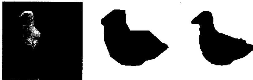
Figure 19.3: Silhouette of a bird by active contour. Left: original image, middle: initial contour, right: final contour (steady state of the snake equation).
