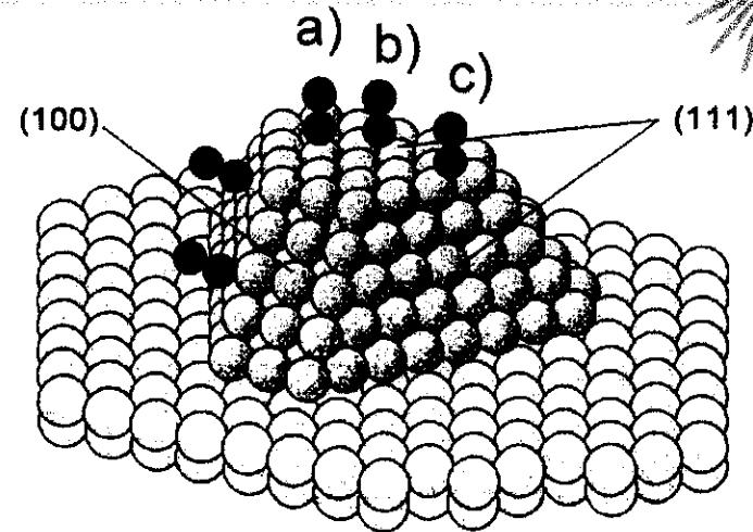
Schematic model of a crystalline Pd particle and the specific adsorption sites of CO.
