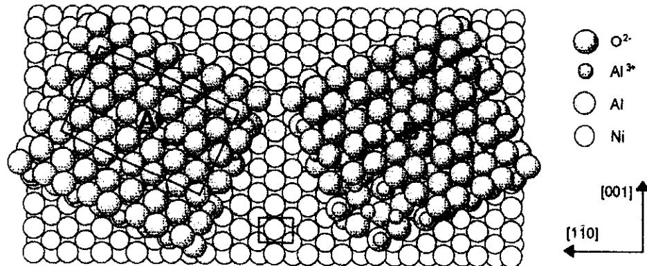
Structure model of  $\text{Al}_2\text{O}_3/\text{NiAl}(110)$ , derived from a distorted g- $\text{Al}_2\text{O}_3$  structure
