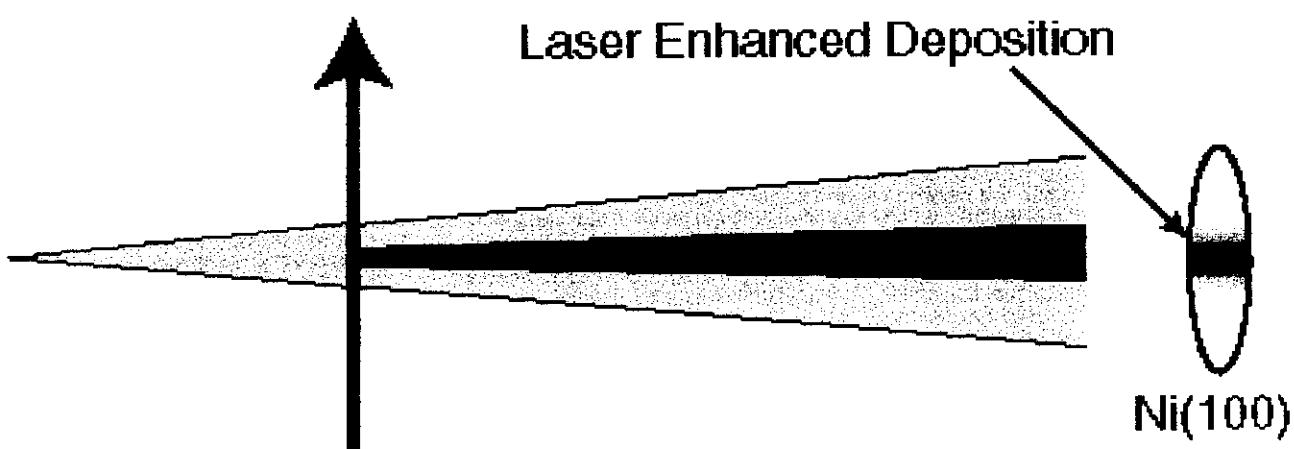
Laser-enhanced deposition is localized on the surface
