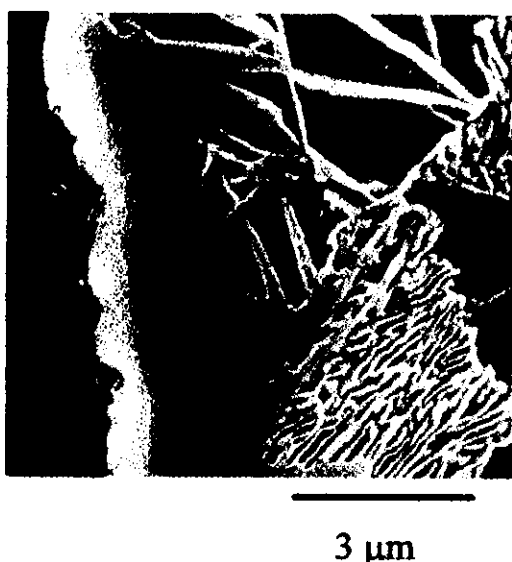
Figure 6. A scanning electron micrograph of a transverse section adjacent to the treated face of the API 5L X-65 6 h plasma-nitrided steel, showing the interaction between the surface ( \gamma' and \epsilon ) nitride layer (E) and the cementite ( Fe_3C ) of a pearlite colony (A).
