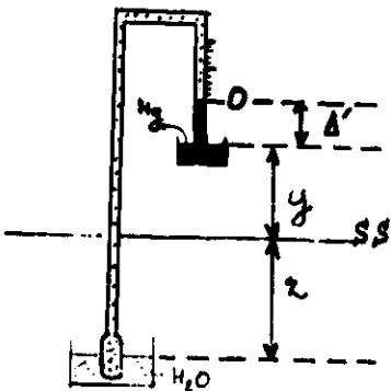
Direct reading of H or h on the scale
