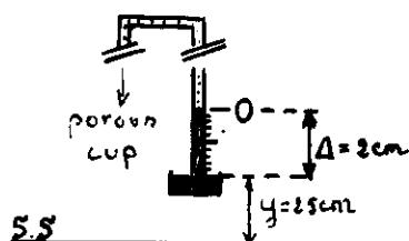
$$\begin{aligned} -12,6x + y + z &= h \\ y &= +12,6x \\ \therefore 0 \text{ or } \Delta &= \frac{y}{12,6} \end{aligned} \quad \left. \begin{array}{l} \text{zero} \\ \text{setting!} \end{array} \right\}$$
