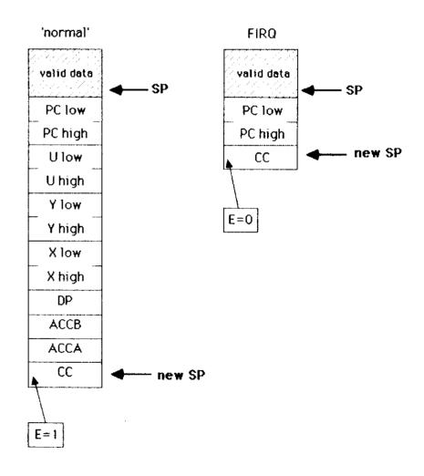
When 'RTI' is executed, CC is pulled first and therefore the CPU will know, if all registers have to be recovered or only the PC in the case of the FIRO
