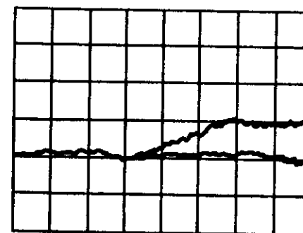
Fig. 2. Oscilloscope trace showing voltage across the Sn-SnO 2 -Sn junction below threshold (lower trace) and the transition from pair-tunneling state to single-particle tunneling state. Horizontal calibration: 0.4 nsec/cm; vertical calibration: 1 mV/cm. H_{\text{external}} = 0 ; T = 1.7^\circ\text{K} .
