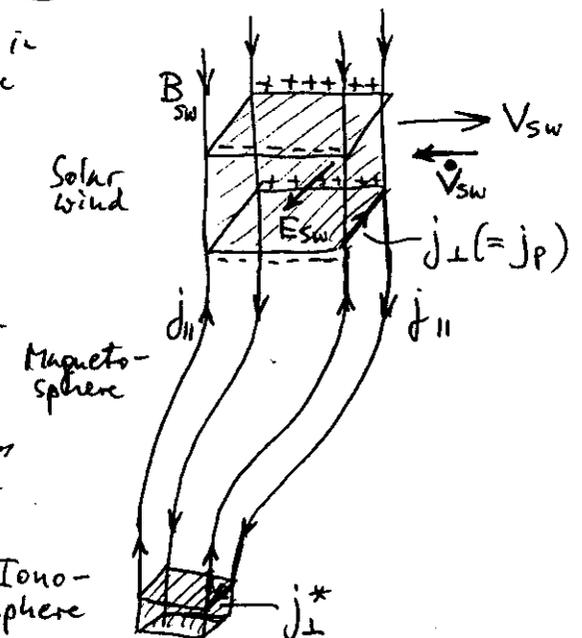
the appearance of a conduction (Pedersen) current  $j_{\perp}^*$  in the ionosphere (closing the current circuit), the appearance of a force  $j_{\perp}^* \times B^*$  on the patch of the ionosphere trying to accelerate it in the direction of solar wind motion, and above all, the appearance of an electric field  $E^*$  in the ionosphere, which is simply the solar wind electric field mapped down along field lines.
