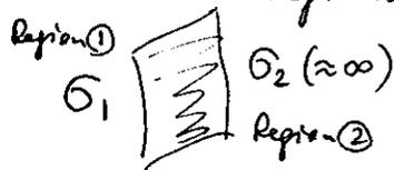
Case II: Two regions of different conductivity  $\sigma$  (e.g., ionosphere and magnetosphere). Separation is not so "sharp" as in Case I, but
