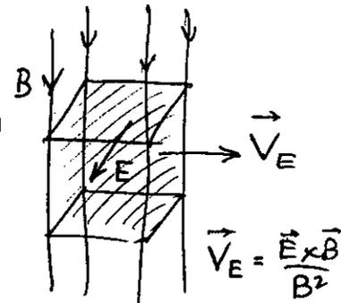
This, however, will lead to an electric field, which in turn will lead to a drift  $\vec{V}_E = \frac{\vec{E} \times \vec{B}}{B^2}$  (bulk motion) which does happen to be in the direction of the original external force  $\vec{f}$ . In other words now the plasma is beginning to react in bulk fashion as we should expect.
