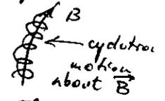
First we define the guiding center system as that frame of reference in which an observer sees the particle execute a closed periodic orbit. If such a frame of reference can be found, we say that the first adiabatic condition is fulfilled, and that frame is unique. The orbits in that Guiding Center System need not be circles (see figure) in the general case. The guiding center (GC) is the centroid of the closed orbit.
