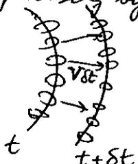
Once the solar wind plasma has been accelerated on the base of the corona, it enters a "cruise mode" of motion away from the sun, in which  $f \approx 0$ ,  $j \neq 0$  and  $\vec{V} = \text{const.}$  It is important to realize that, as viewed from a system fixed to the Earth, the solar wind has an electric field
