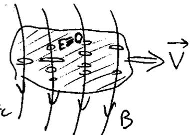
Therefore, if a point a field line with probe particles in that frame, these particles will remain on that field line in that frame. Therefore, the field line is moving with the plasma!
