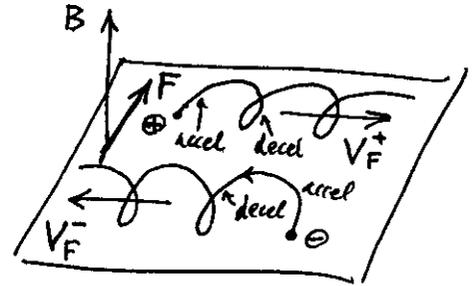
If still does not depend on energy, but it does depend on electric charge. In response to an external force, the particles respond with a transverse drift, with positive and negative particles going in opposite directions. This will lead to an electric current of density
