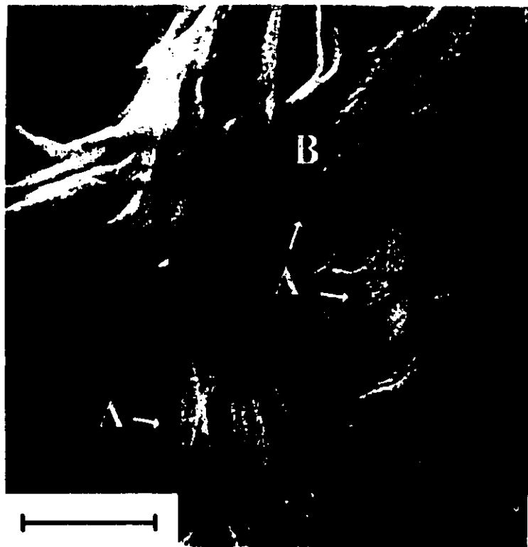
Figure 3.19. Scanning electron micrograph illustrating the lamellar structure of a melt-crystallized spherulitic polyethylene. The cavernous texture enabling the lamellae to be seen in depth arises as follows: the lower-molecular-weight material segregates on crystallization in separate lamellar packets, which can be removed subsequently by selective dissolution treatment (after Winram et al. 117 ).
