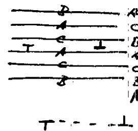
Shift all atoms in the upper section relative to those in lower section; parallel to (111) plane in such a direction that the atoms on the lowest plane of the upper section B  $\rightarrow$  C
