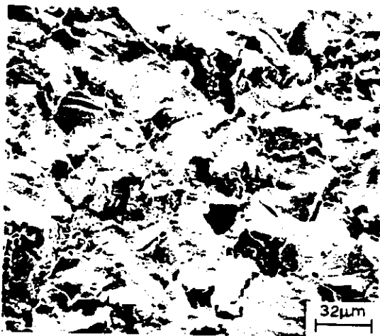
23 Surface cracks in LRO-1 specimen fractured in tension at 1000°C, showing nodules formed by dynamic crystallization localized along grain boundaries
