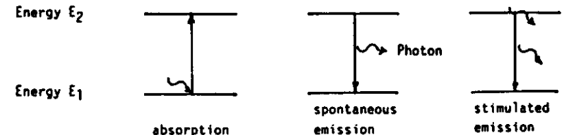
Fig. 13. Energy level diagram illustrating absorption (a), spontaneous emission (b) and stimulated emission (c).
