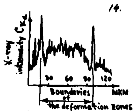
Carbon distribution on a deformed bronze surface irradiated by 40 \text{ keV Ar}^+ ions.
