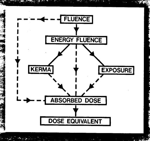
An equipment for measuring absorbed dose via temperature changes caused by irradiation of a suitable material is called a calorimeter. It is clear that such a dosemeter is of no practical use in routine radiotherapy and even less in radiation protection measurements. Therefore, other ways had to be found and historically have been taken to measure absorbed dose to water. This way is based on the property of radiation to ionize air and leads to the quantity Exposure (X) and its unit Roentgen (R).
