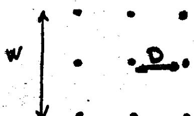
The recording grid spacing  $D$  determines the spatial sampling rate, and affects the higher spatial frequencies, whereas the total width  $W$  affects the lower spatial frequencies.
