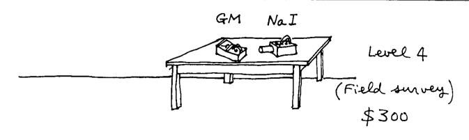
Instrumentation for measuring radioactivity in food.
