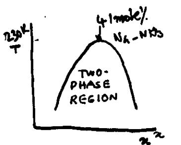
Possibility of phase segregation in composition-controlled metal insulator transition.
