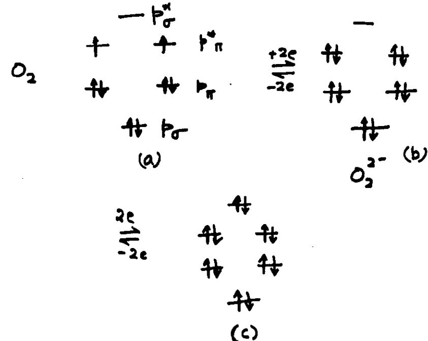
TOP of valence band anti-bonding in character. holes in valence band creates bonds. O-O bonds vs Cu-O bonds. If  $\text{Cu}^{2+}$ ; Cu-O bonds. If  $\text{Cu}^{4+}$  O-O bonds?
