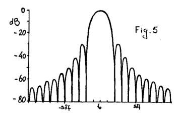
The mainlobe is 48f, double the width of the rectangular window. Sidelobes are more attenuated, and the fall off rate is much faster than for BoxCar weighting. This means that the 60dB bandwidth is much narrower, giving better selectivity. The ripple is only 1.4 dB.
