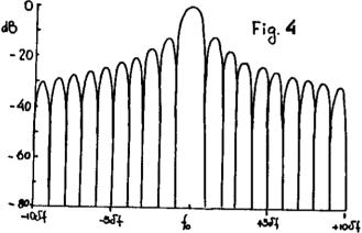
The filter has a mainlobe which is twice the width of the line-filter spacing (  $\delta f = 2\pi n/T$  ) and an INFINITE number of sidelobes with widths equal to the line filter spacing. For the analysis of deterministic/harmonic signals this is a poor filter because it has:
