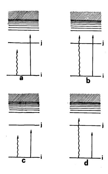
FIGURE 1. Schematic energy representations of the processes of PEAC.
