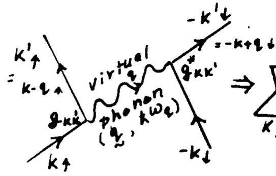
$$\Rightarrow \int_{k,q} \frac{|g_{kk'}|^2 \hbar \omega_q}{(\epsilon_{k-q} - \epsilon_k)^2 - (\hbar \omega_q)^2} C_{-k+q\downarrow}^\dagger C_{k+q\uparrow}^\dagger C_{k\uparrow} C_{-k\downarrow}$$
