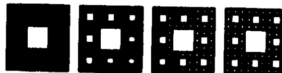
FIGURE 2.16: Construction of the Sierpinski carpet. The initiator is a square and the generator (shown on the left-hand side) is made of N = 8 squares. They are obtained by contractions of ratio r = 1/3 . The right-hand side of the figure shows the fourth construction stage. The similarity dimension is D = \ln 8 / \ln 3 = 1.89 \dots
