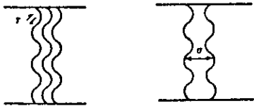
Figure 8.30. (a) Brittle failure in torsion. (b) Longitudinal failure in uniaxial compression between unlubricated platens. (c) Fiber buckling modes in uniaxial composite subject to uniaxial compression parallel to the fiber direction.
