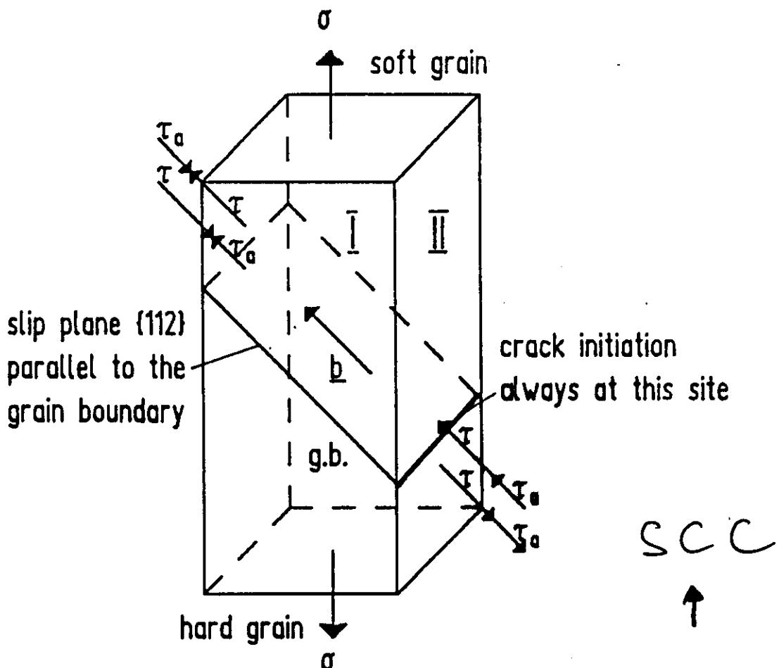
sensitive orientations for the nucleation of cracks by
