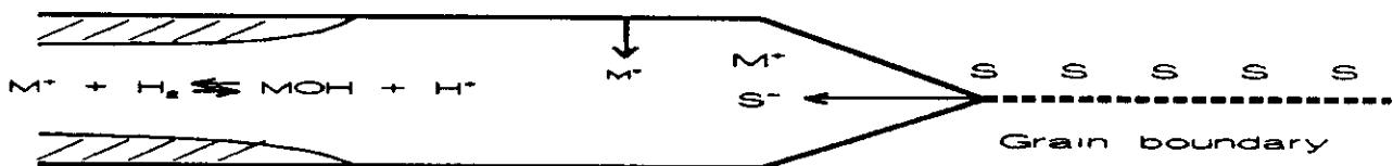
Reactions at crack walls, transport of ions to and from the crack tip change in pH and concentration influence the potential at the electrochemical double layer at the crack tip.
