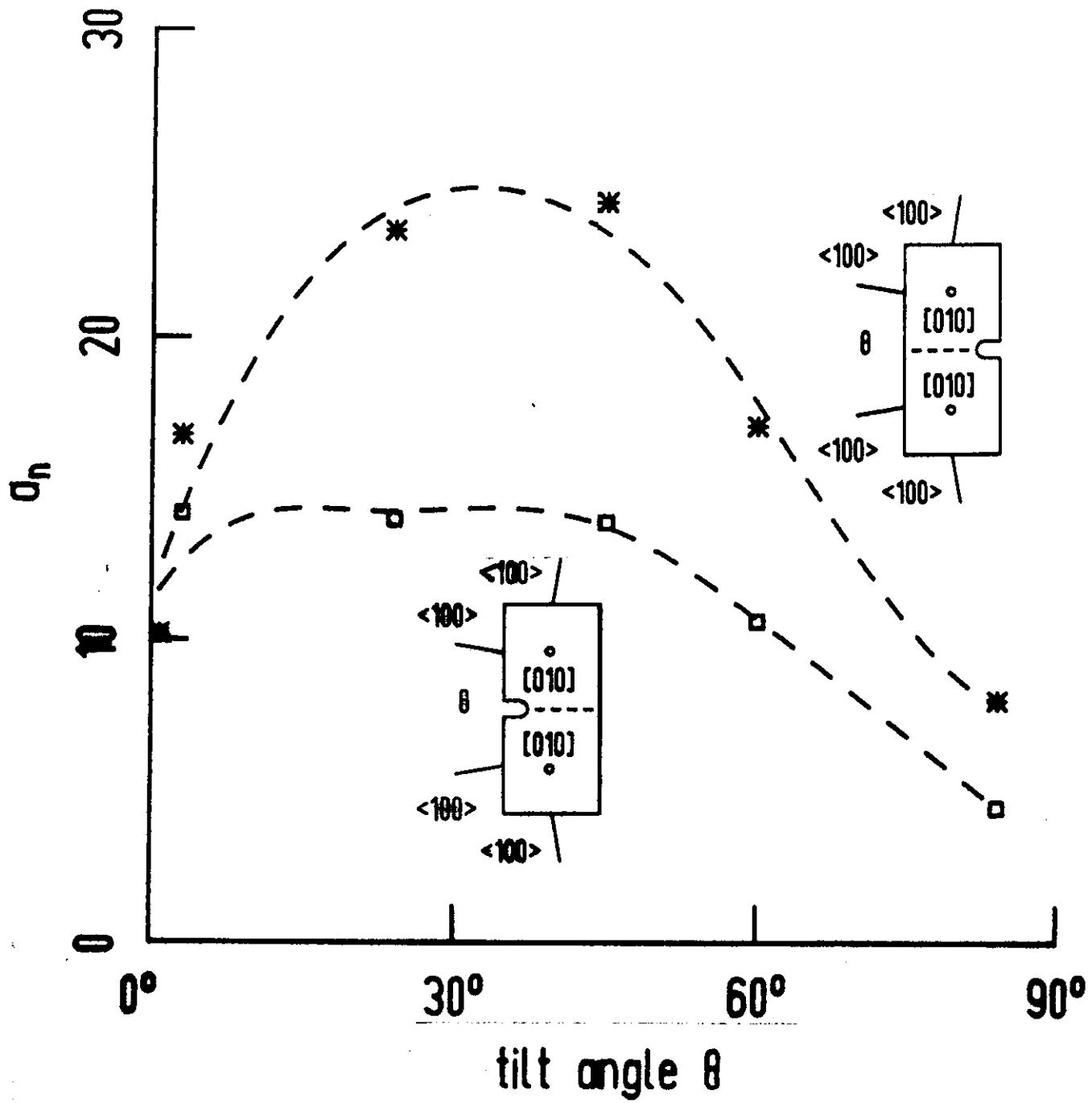
\* and □ are measurements for the same boundary, only the slip distribution at the crack tip is different.
